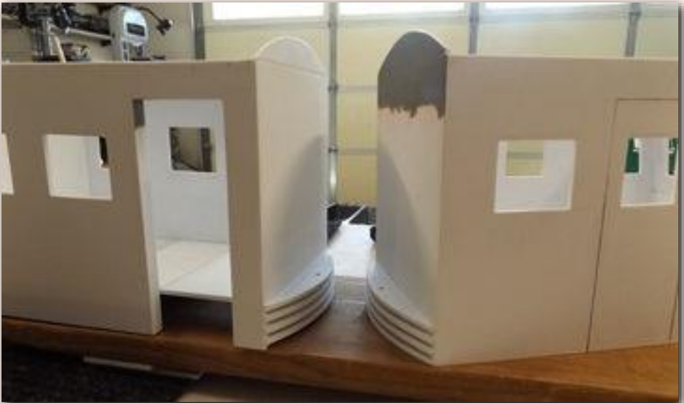
This photo shows the couplers that will connect the two sections together and allow the two sections to rotate.
