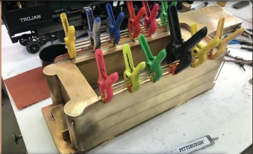
Though this loco was an oil burner it had a fence on top of the tender. Here it is being attached
