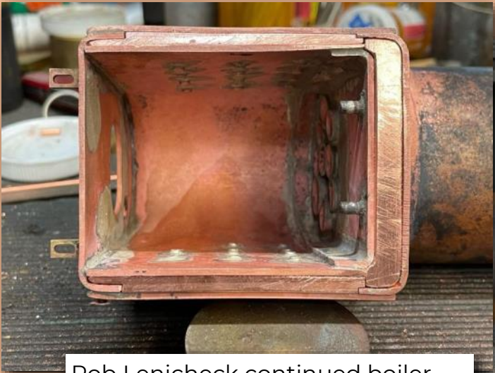
Rob Lenicheck continued boiler work on his Darjeeling. Closing up the gaps at the bottom of the firebox is always a puzzle
