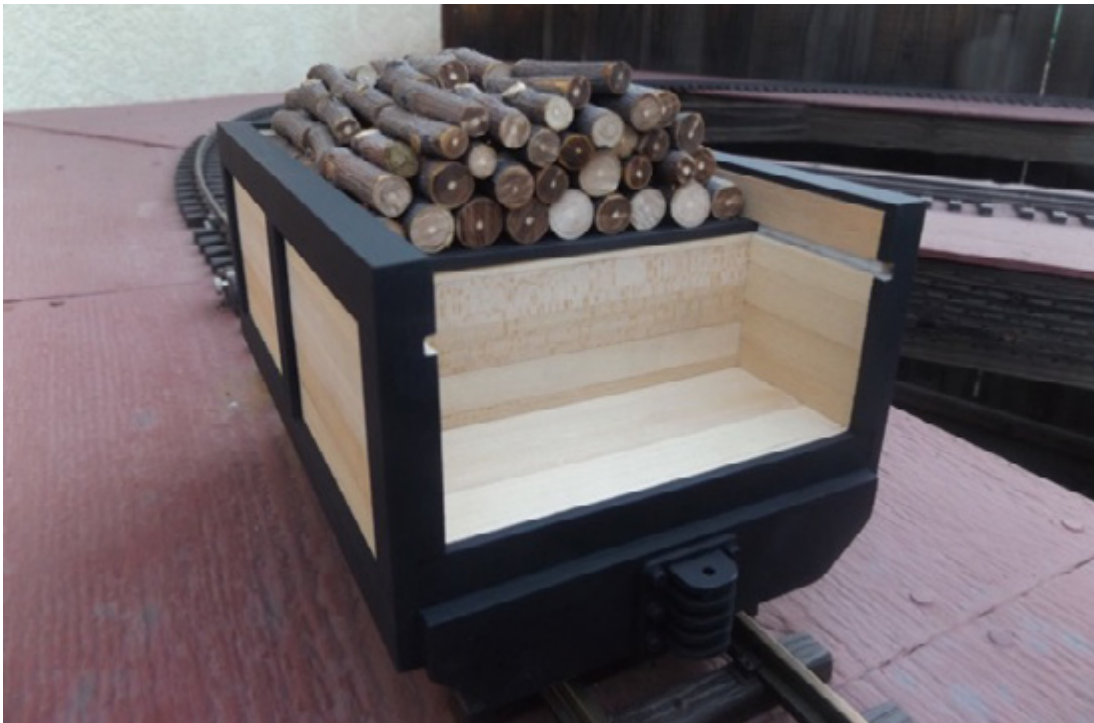
Photo #1987 - Shows inside of tender with wood planking completed
