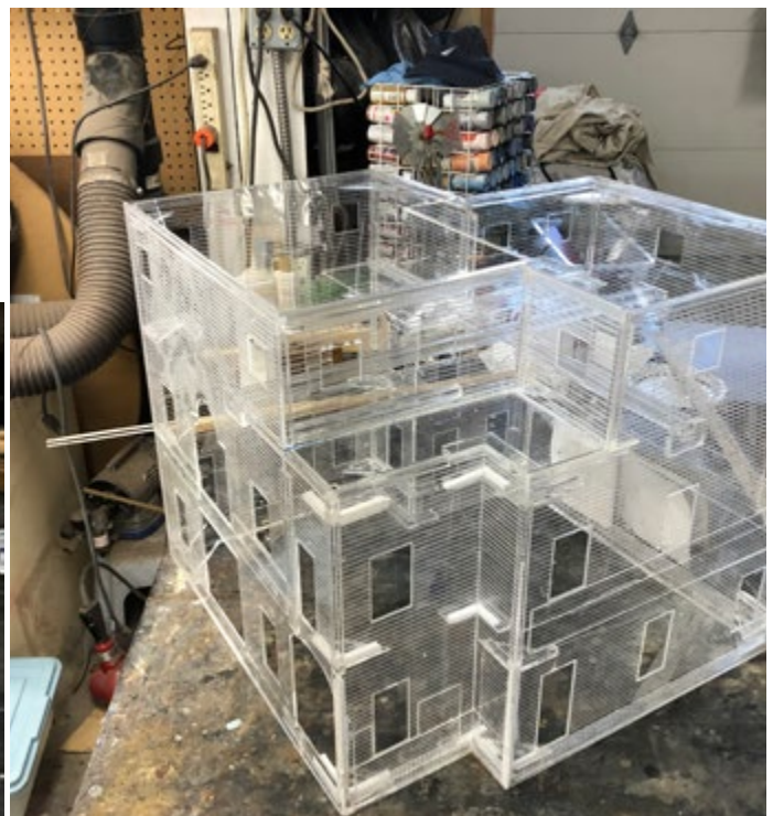
Once all the bracing is installed, the structure is ready to paint. To glue acrylic a solvent type of cement is used to weld the plastic together. Solvent cement will dissolve paint so, one must cement everything together before painting.
