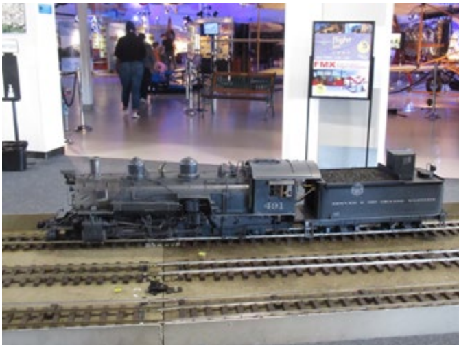
Rob Lenicheck really does have an engine that is not coal fired. This one uses butane and is an Accucraft K-37.
