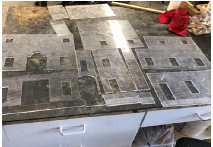
The walls were cut out of 1/8" thick acrylic. During the same process the brick and planking line were engraved. With laser cutters, the difference between engraving and cutting is the power setting.
