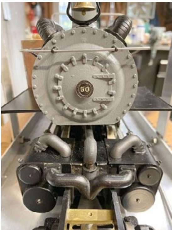
Smoke box door and various pipes are 3D printed in metal
