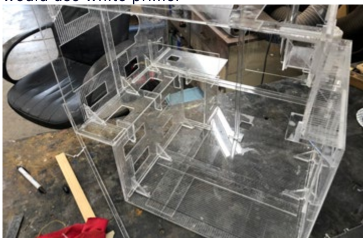
Here the walls have been assembled. A piece of square stock is used in the corners for reinforcing. Special corner braces have been made to ensure the walls are square, during construction.
