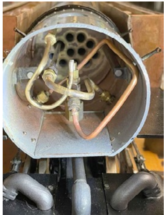
A view into the smoke box:
