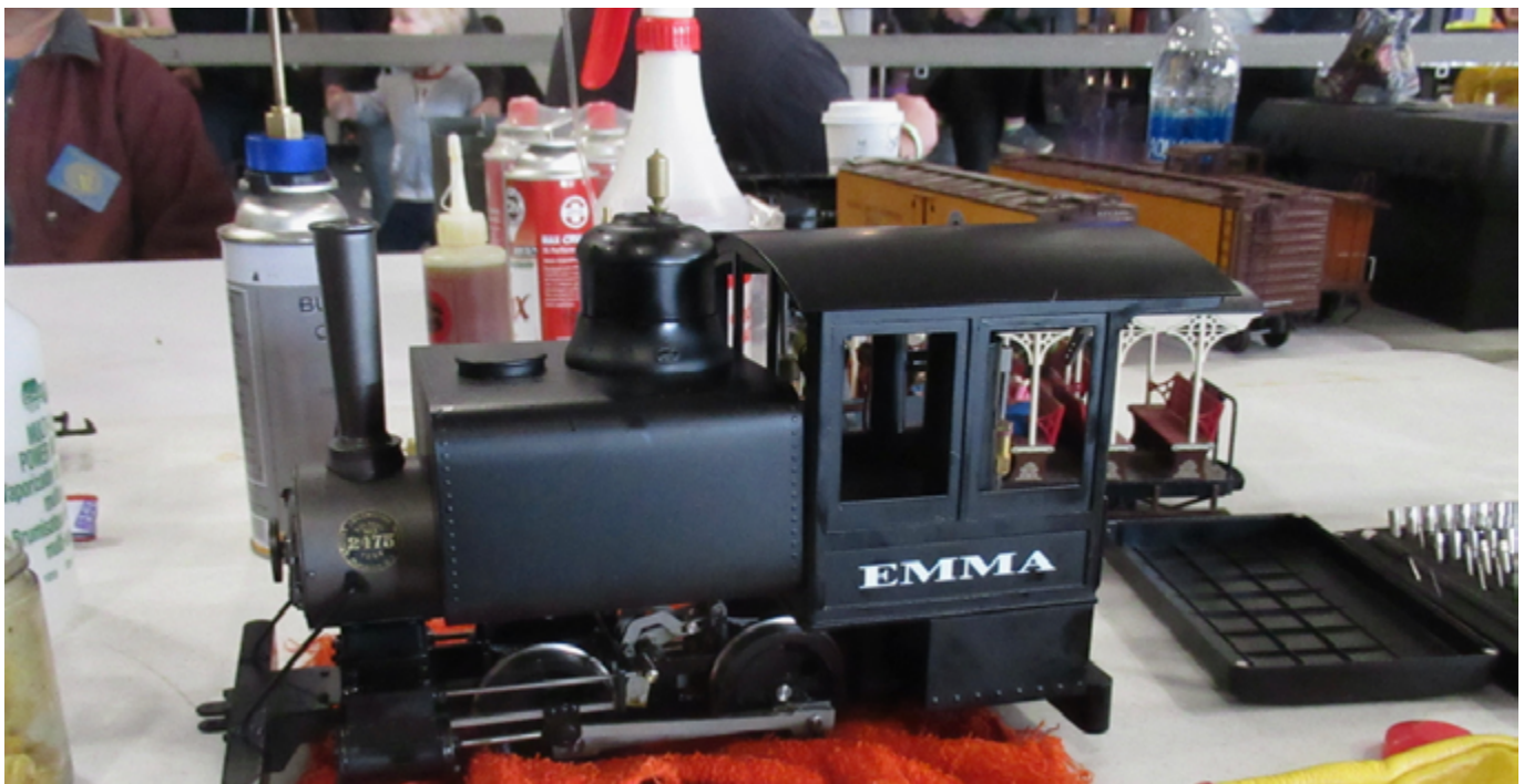
Emma, is an Accucraft product that is 7/8ths scale. It is a model of a Brooks industrial 0-4-OT. Brooks Locomotive Works of Dunkirk, New York merged to become the American Locomotive Company, or ALCO.
