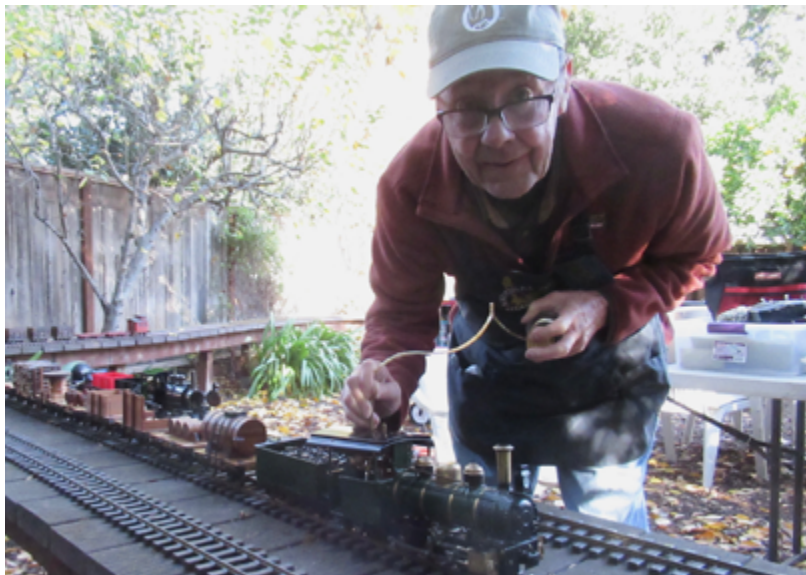
Jim Goss is fueling his Roundhouse Fowler with his special tube adapter. He is about to pull many kit built Ozark cars.
