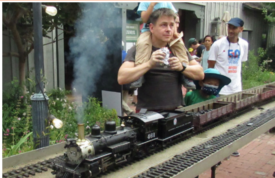
Steve Heselton was one of the first BAGRS live steam members to popularize coal firing. Here is his Accucraft K-27 2-8-4 that was converted to coal. It's a big engine! Steve has placed "dirty" coal in the fire box to create more smoke and more smell.
